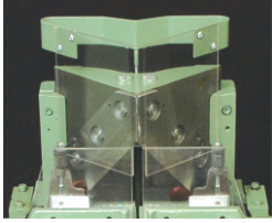
Safety Guard: designed to protect the operator from highly sharp knives
