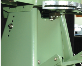
Spring Adjuster: equipped with 5 level of footpedal spring adjuster
